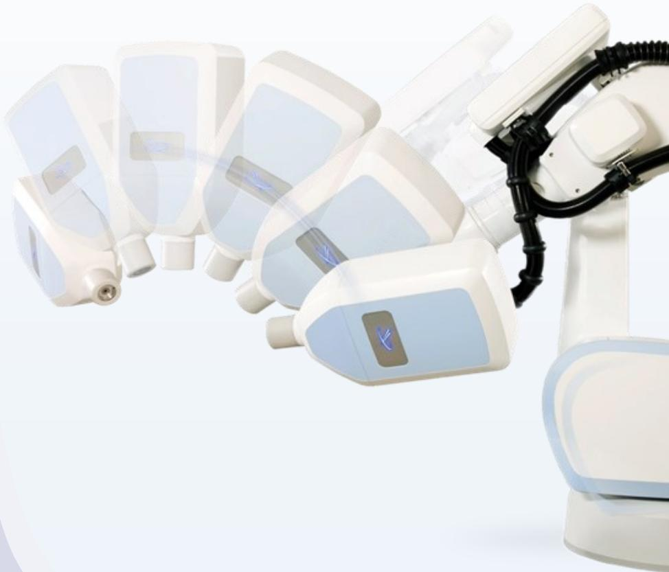
The CyberKnife system is based on a small linear accelerator (LINAC) mounted on a flexible robotic arm. With robotic technology radiotherapy can be focused on to a desired point within an accuracy of even 0.5 millimeter from several different directions.
